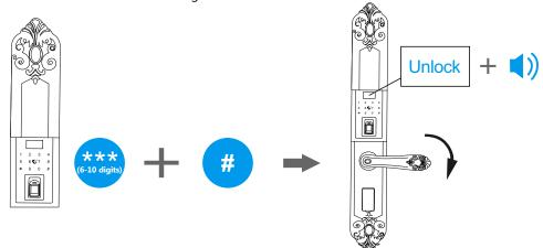
When inputting a wrong password for 3 times, the lock will be locked for 5 minutes. During the 5 minutes, the lock cannot be activated and all operations are not available. After that, the lock returns to normal state.
